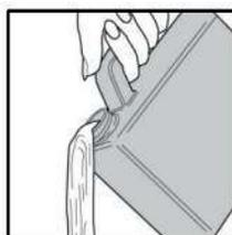
The container can then be removed and emptied as shown. Replace the container back into the dehumidifier with the outlet on the left hand side and gently close the door.
